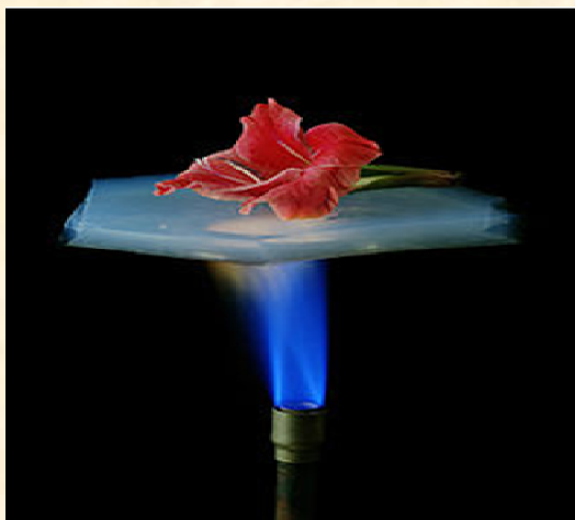
A flower is on a piece of aerogel which is suspended over a Bunsen burner. Aerogel has excellent insulating properties, and the flower is protected from the flame
